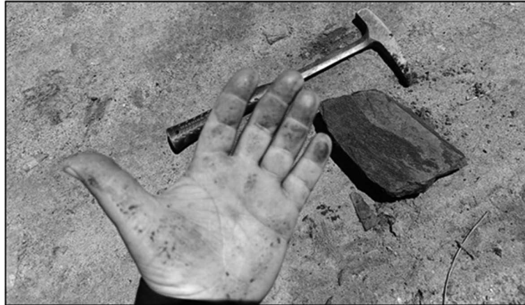
Figure 9-2: Graphite phyllite sample exhibiting a dark color and a shiny appearance, leaving pigmentation upon contact with the hand
