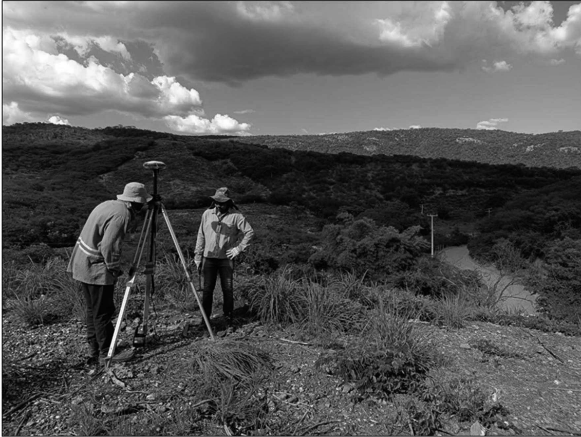
Figure 9-12: Details on the use of the Geodetic GPS RTK (Trimble SP60) for acquiring cadastral planialtimetric data in the mineral research area under ANM Process No. 870.512/2019
