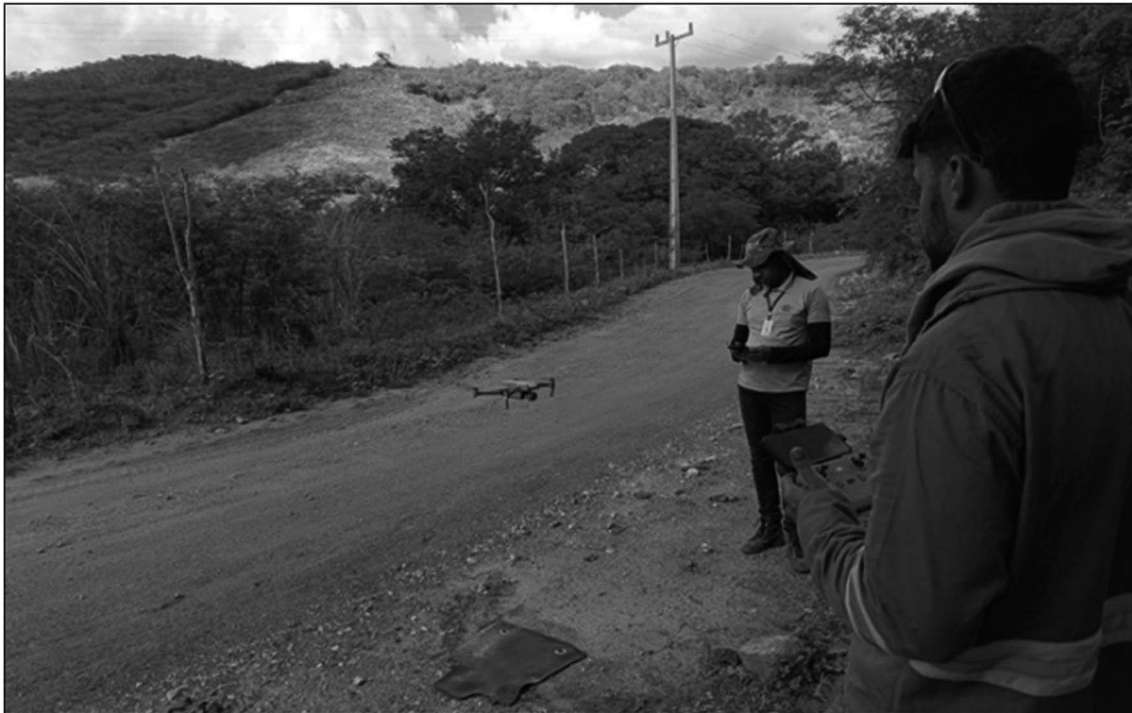
Figure 9-10: Execution of an aerial photogrammetric survey in the mineral research area under ANM Process No. 870.512/2019
